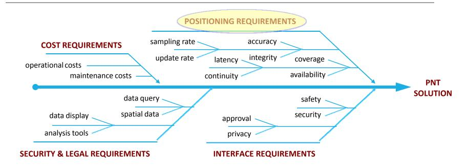
user requirements can be listed in a "fish plot", in which four basic categories can be recognized
